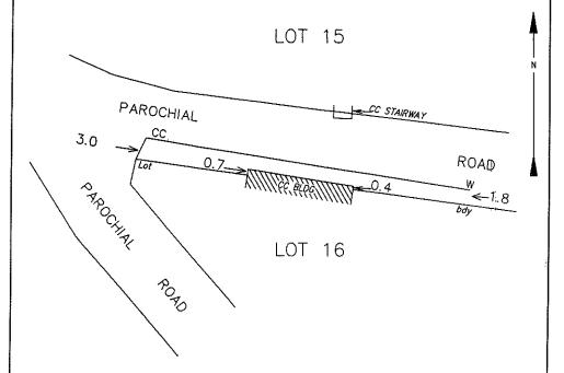
Remarks 1: Measurements are in metres. 2. A part of the concrete building on lot 16 is encroaching on the parochial road to the north by 0.4 to 0. metres. The lot is incorrectly fenced on the northern boundary, the concrewall is encroaching on the parochial road by 1.8 to 3.0 metres. 3. A part of the staircase on Lot 15 is encroaching on the parochial road to the south by 0.7 to 0.9 metres
